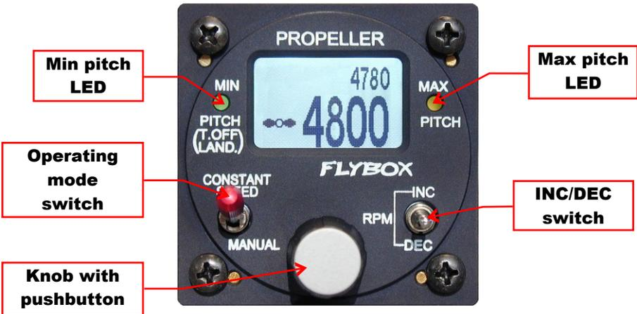
The knob with pushbutton can be rotated (for example to increment or decrement the RPM) or pressed like a pushbutton (for example to enter in the menu or in the various settings).
