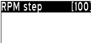
**RPM step:** set the minimum step when changing the RPM with the knob or the INC/DEC switch. The step value can be 10,25,50 or 100 RPM.
