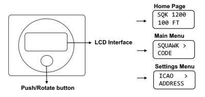
On power ON, the LCD interface will display the company name "LEVIL AVIATION", firmware and serial number, followed by the Home Page. To navigate between the screen modes, use the button as follows:
